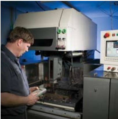
KMC's toolmaking equipment includes several wire EDM machines.
