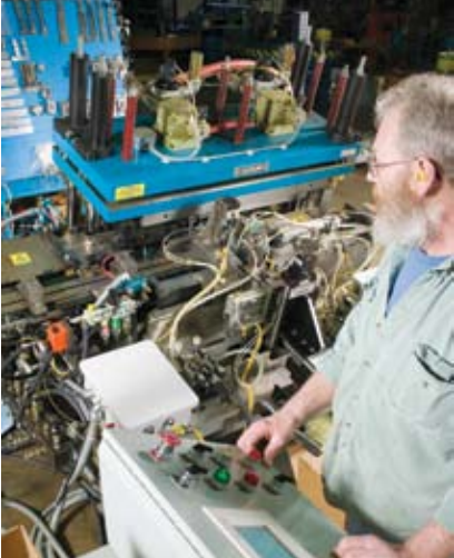
KMC develops unique metal forming equipment, such as this multi-process production machine for extruded-cushion clamps.
