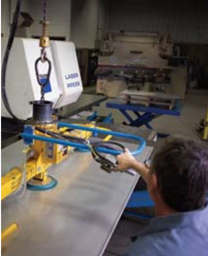
Laser presses, which don't require hard tooling, are used extensively for rapid-response prototyping.
