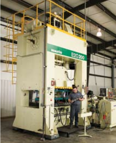
This 200-ton unit is one of many punch presses spread among KMC's multiple manufacturing facilities.
